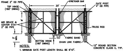
2. CHAIN LINK FABRIC TO MATCH FABRIC ON CHAIN LINK FENCE.
