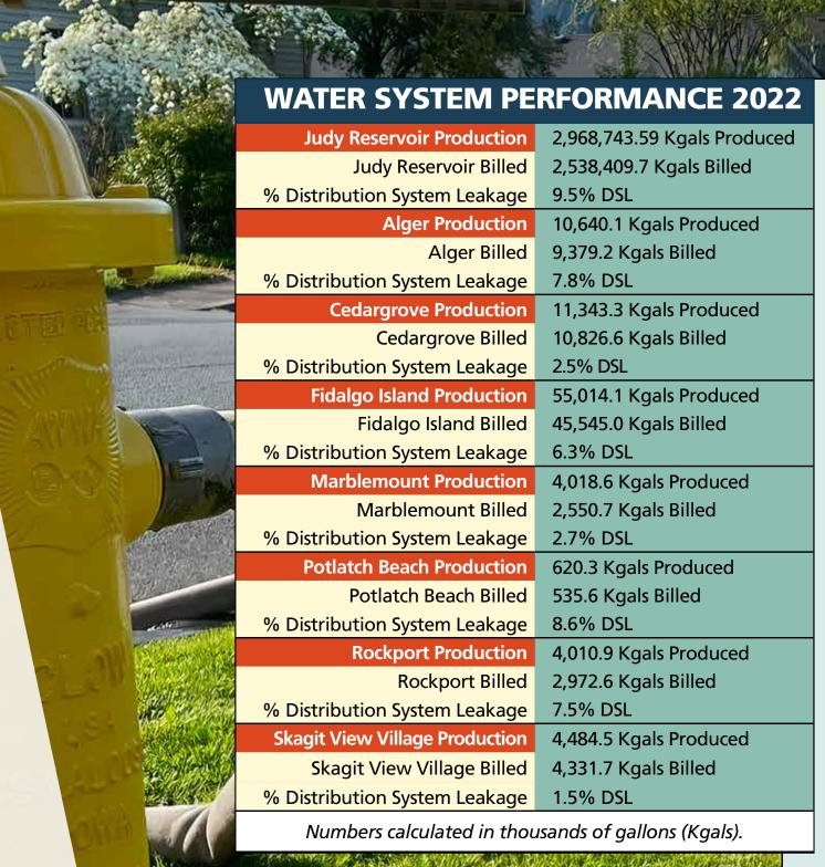
The chart at the left reports each system's water production performance for 2022. All water that is not authorized consumption is considered distribution system leakage (DSL). Some examples of water use considered leakage include: water main breaks, theft, meter inaccuracies, meter reading errors, data collection, and calculation errors.
