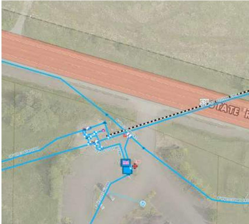
**Existing Water Source No. 2:** Existing 2-inch flushing assembly located in the NE Corner of the Slavic Church parcel.
